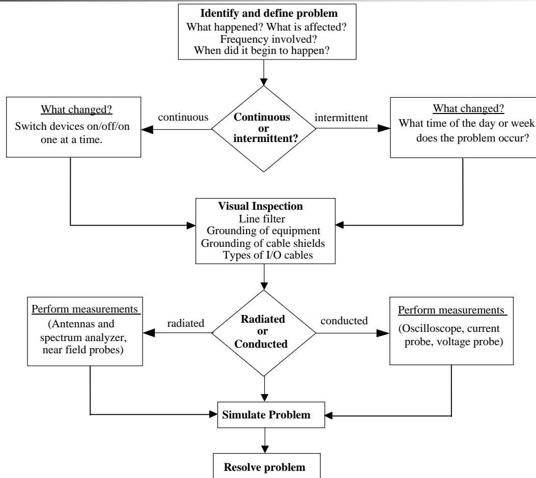
Figure 8.5 Systematic approach to detecting and locating problems
